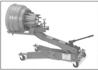
Eliminate seal damage when installing inboard drums
